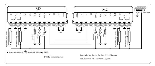
DC12V Commom Power Two Units Interlocked for Two Doors Diagram
